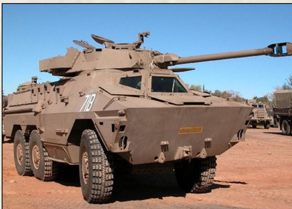
FIRE SUPPORT: A Ratel-90, armed with its 90 mm gun.
