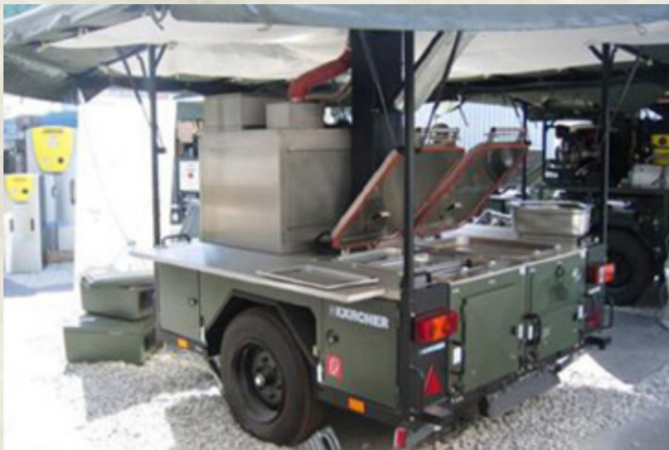
COOKING IN THE FIELD: The 250-man mobile field kitchen was a nifty piece of equipment. Many of the bush bases used these and you could cook just about anything in them - even bake bread.
