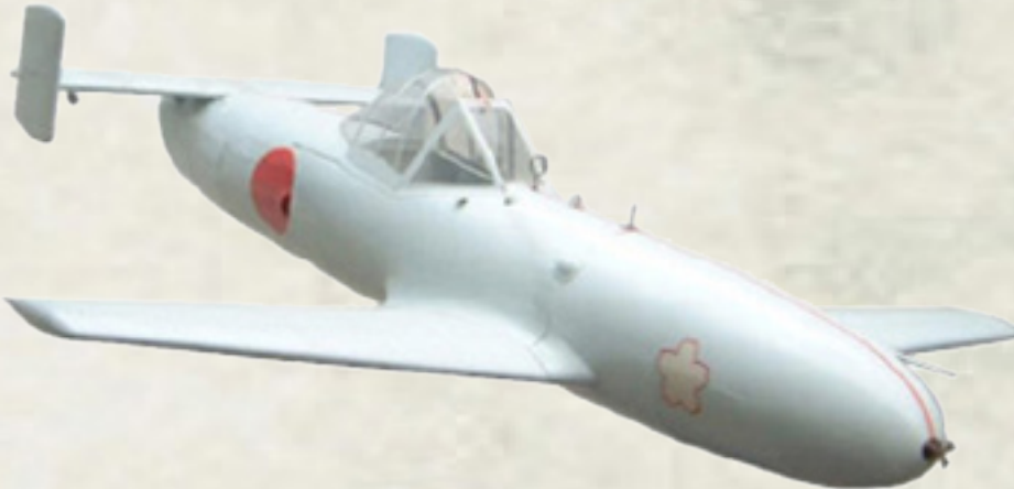
FLYING BOMB: Japanese Yokosuka MXY-7 Ohka ("cherry blossom"), a specially built rocket-powered kamikaze aircraft used towards the end of the war. The U.S. called them Baka Bombs ("idiot bombs").
