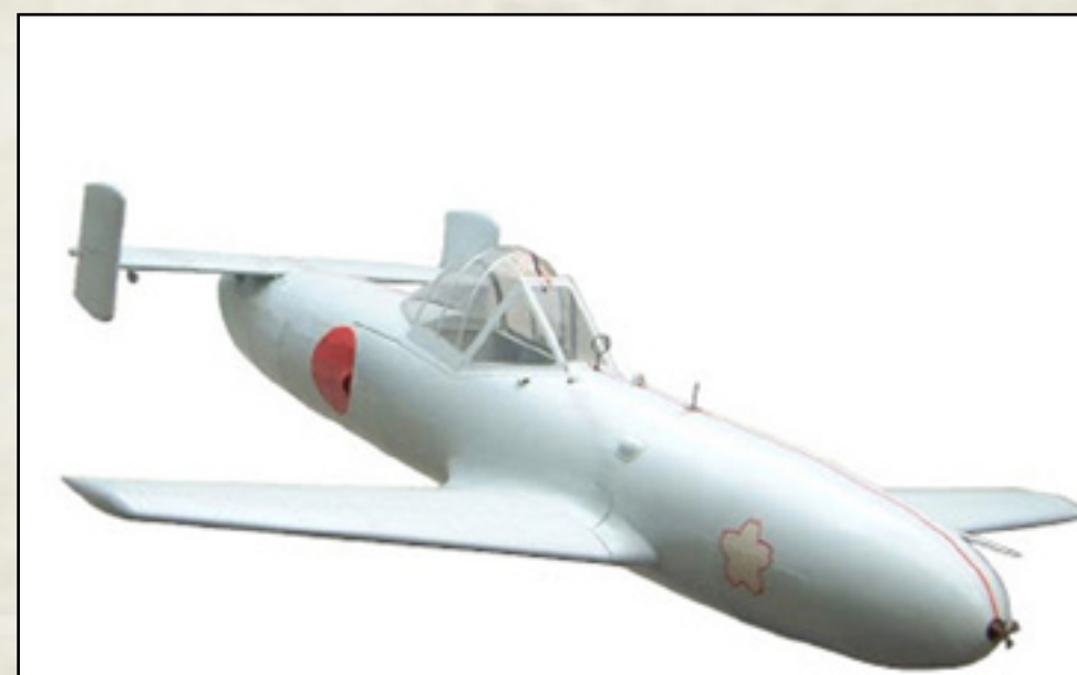
FLYING BOMB: Japanese Yokosuka MXY-7 Ohka ("cherry blossom"), a specially built rocket-powered kamikaze aircraft used towards the end of the war. The U.S. called them Baka Bombs ("idiot bombs").
