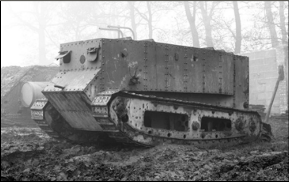
PROTOTYPE: "Little Willie" was the first prototype tank. It carried a crew of three and could travel as fast as 4.8 km/h.
